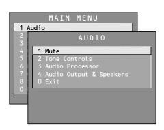
**Second Audio Program (SAP)** Plays the program's audio in a second language, if one is available. The TV displays the word SAP when you tune to a program that is broadcast with SAP information. SAP audio is broadcast in mono. SAP is also used to broadcast a program's audio with descriptions of the video for the visually impaired.
